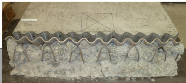
Due to the special shape of the sinusoidal consoles and their opposite arrangement, the introduced forces can be distributed very uniformly in the length direction of the profile.
